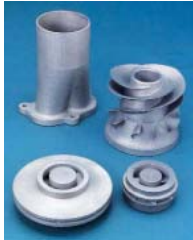
Testing the metal: These prototype rocket engine parts were made by laser-binding metal alloys, then baking them in a furnace.
